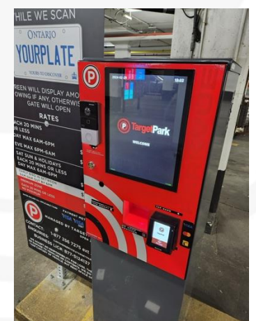
Villa Door Station installed on white label payment station. User can communicate with a control center for payment issues etc.
